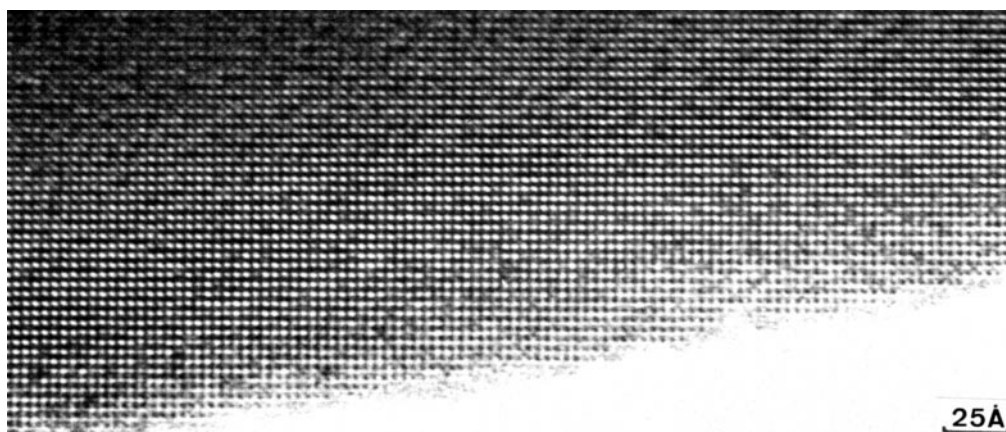
FIG. 7. HRTEM image of a PTB crystal projected along [001] . Partial occupancy of the tunnels in the perovskite lattice can be seen, especially in the thinner region of the crystal.
